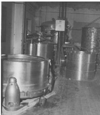
Noseda Salvadore Italian fibers dyeing machine and the Swiss "Jigger" dyeing machine
