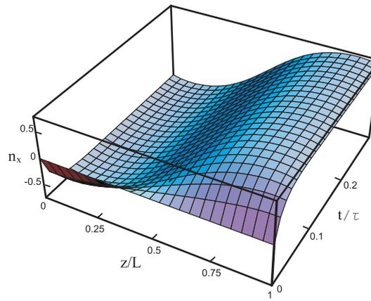
**Fig.6.** Three-dimensional time and space dependence of the director's x component after switching the laser radiation "on"; for homeotropic oriented cells in the case of the generalized problem.
