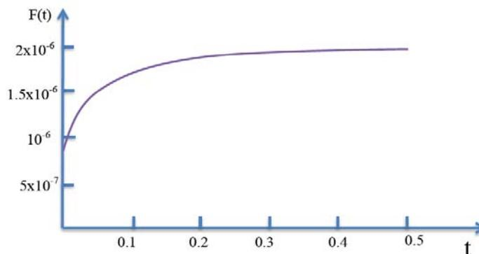
**Fig 8.** Deformation free energy of the hybrid oriented liquid crystal cells after switching the laser radiation "on".
