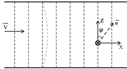
Fig.2. Director profile in a homeotropic oriented cell with nematic LC.
