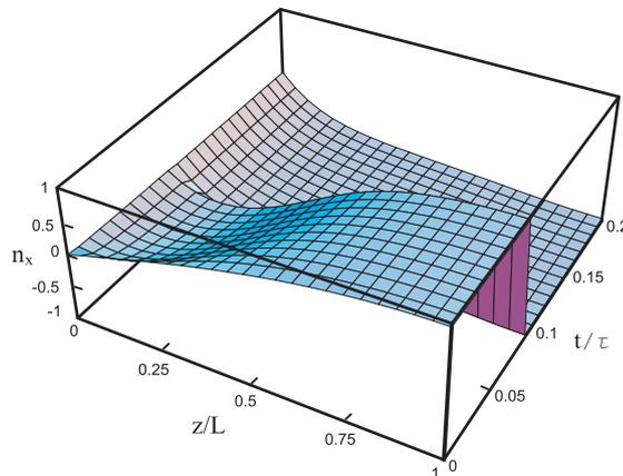
**Fig.10.** Three-dimensional time and space dependence of the director's x component after switching the laser radiation “on”; for hybrid oriented cells in the case of the generalized problem.
