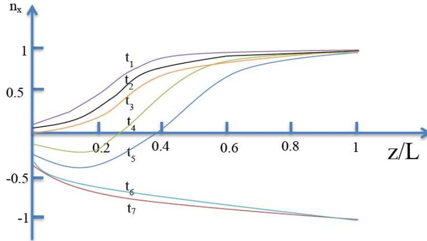
**Fig.9.** Profile of the director's x component ( $n_x$ ) for different times ( $t_j$ ) after switching the laser radiation “on” for hybrid oriented cells in the case of the generalized problem ( $t_1 = 0$  sec,  $t_2 = 3.8 \cdot 10^{-5}$  sec,  $t_3 = 1.14 \cdot 10^{-4}$  sec,  $t_4 = 1.9 \cdot 10^{-4}$  sec,  $t_5 = 3.8 \cdot 10^{-4}$  sec,  $t_6 = 1.14 \cdot 10^{-3}$  sec,  $t_7 = 3.8 \cdot 10^{-3}$  sec). Reversal time is  $t_r = 0.68 \cdot 10^{-3}$  sec.
