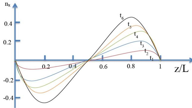
**Fig. 5.** Profile of the director’s x component ( $n_x$ ) for different times ( $t_j$ ) after switching the laser radiation “on” for homeotropic oriented cell with an approximation of strong anchoring. ( $t_1 = 0 \text{ sec}$ ,  $t_2 = 2.28 \cdot 10^{-5} \text{ sec}$ ,  $t_3 = 0.68 \cdot 10^{-4} \text{ sec}$ ,  $t_4 = 1.14 \cdot 10^{-4} \text{ sec}$ ,  $t_5 = 2.28 \cdot 10^{-4} \text{ sec}$ ,  $t_6 = 2.28 \cdot 10^{-3} \text{ sec}$ ).
