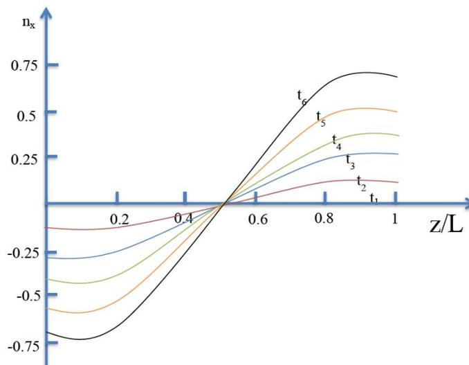
**Fig.7.** Profile of the director's x component ( $n_x$ ) for different times ( $t_i$ ) after switching the laser radiation "on" for homeotropic oriented cell in the case of the generalized problem. ( $t_1 = 0$  sec,  $t_2 = 2.28 \cdot 10^{-5}$  sec,  $t_3 = 0.68 \cdot 10^{-4}$  sec,  $t_4 = 1.14 \cdot 10^{-4}$  sec,  $t_5 = 2.28 \cdot 10^{-4}$  sec,  $t_6 = 2.28 \cdot 10^{-3}$  sec).
