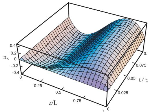
**Fig.4.** Three-dimensional time and space dependence of the director’s x component after switching the laser radiation “on”; for homeotropic oriented cells with an approximation of strong anchoring.
