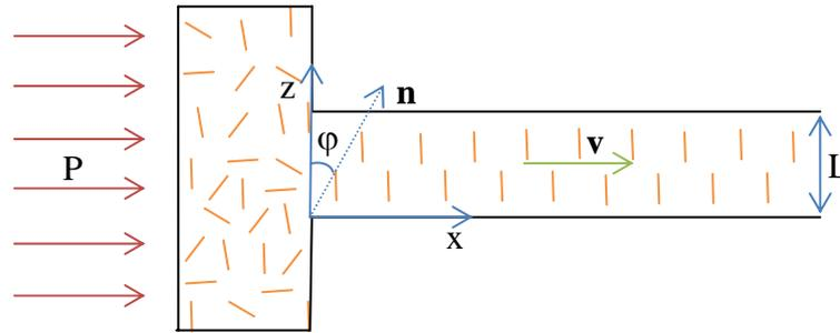
**Fig.1.** Considered cell:  $P$  is the radiation intensity,  $\mathbf{v}$  is the flow velocity,  $L$  is the thickness of capillary and  $\mathbf{n}$  is the NLC director.
